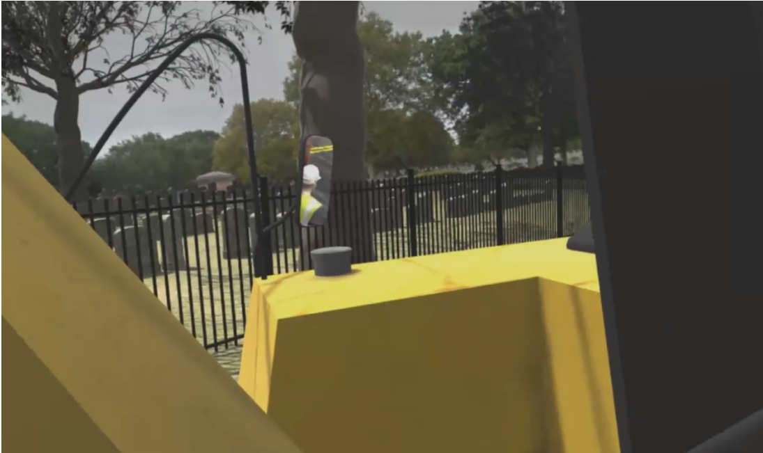
An operators view of an excavator mirror, showing line of site of a worker on the ground, through HTC Vive
